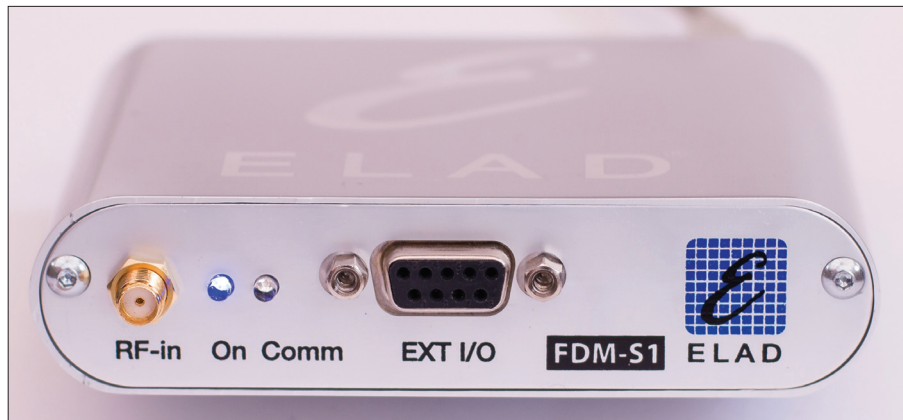
The ELAD FDM-S1 direct sampling SDR receiver.
